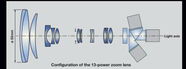
The wide-angle zoom lens that gained high popularity in the HVX200 Series has been reduced in size, lightened, and further widened in this 13x zoom lens. The lens structure combines 13 lens elements in 10 groups, with 3 aspherical lenses. The diameter of the front lens element has been reduced from 67 to 53.2 mm, while still achieving a 28mm wide angle (35mm equivalent), the widest of the class.\*
