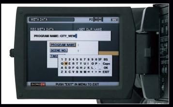
The P2 cam records each recording as a clip (file) and automatically attaches a thumbnail image and file information to it. To preview a clip on the LCD monitor or to check clip data, simply choose the clip you want from the list of thumbnails. It also supports metadata input using a software keyboard.
